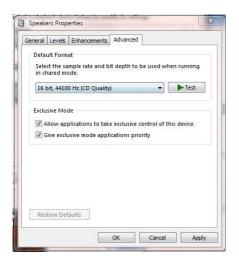
To avoid the interface unexpectedly activating your radios PTT, Windows must be configured so that "system sounds" are played via your original soundcard and not via the DataLink soundcard.
